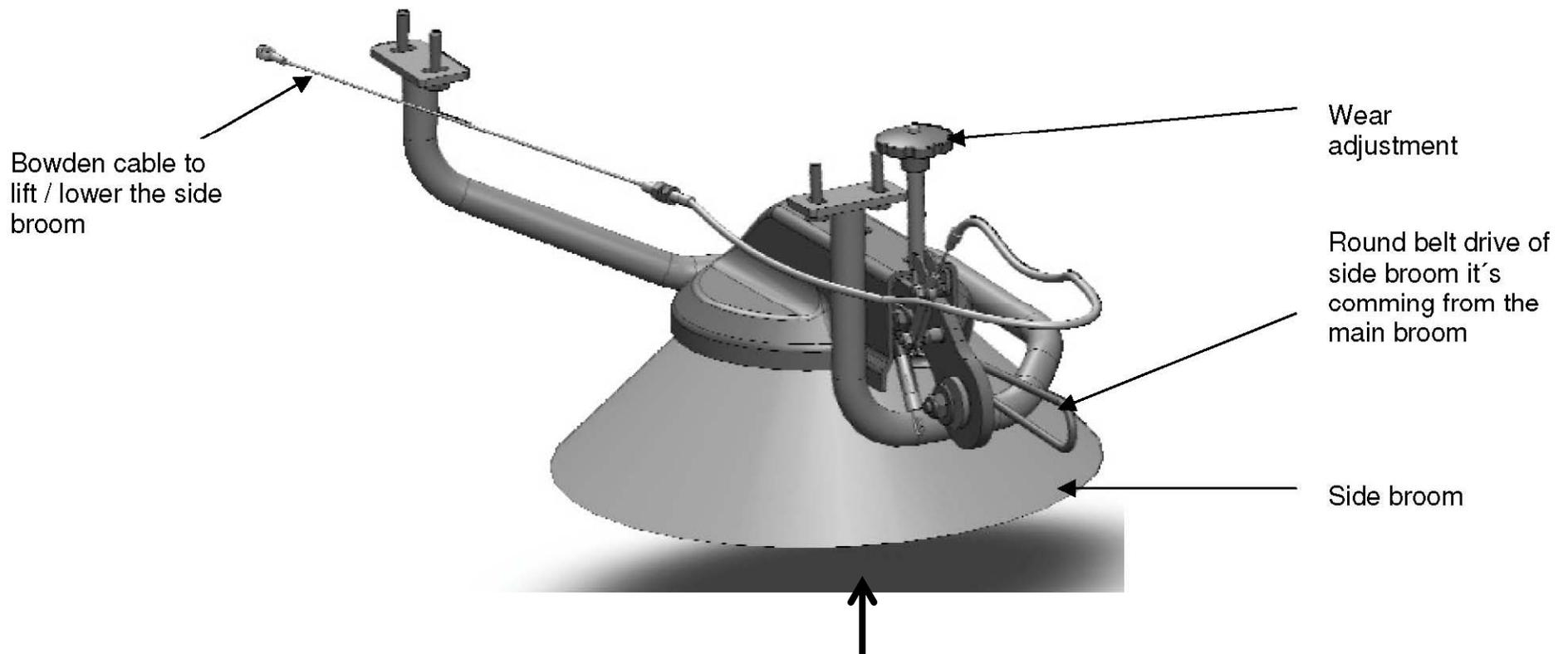
On the underside of the broom block there are hexagonal nuts and washers for mounting the side broom.
