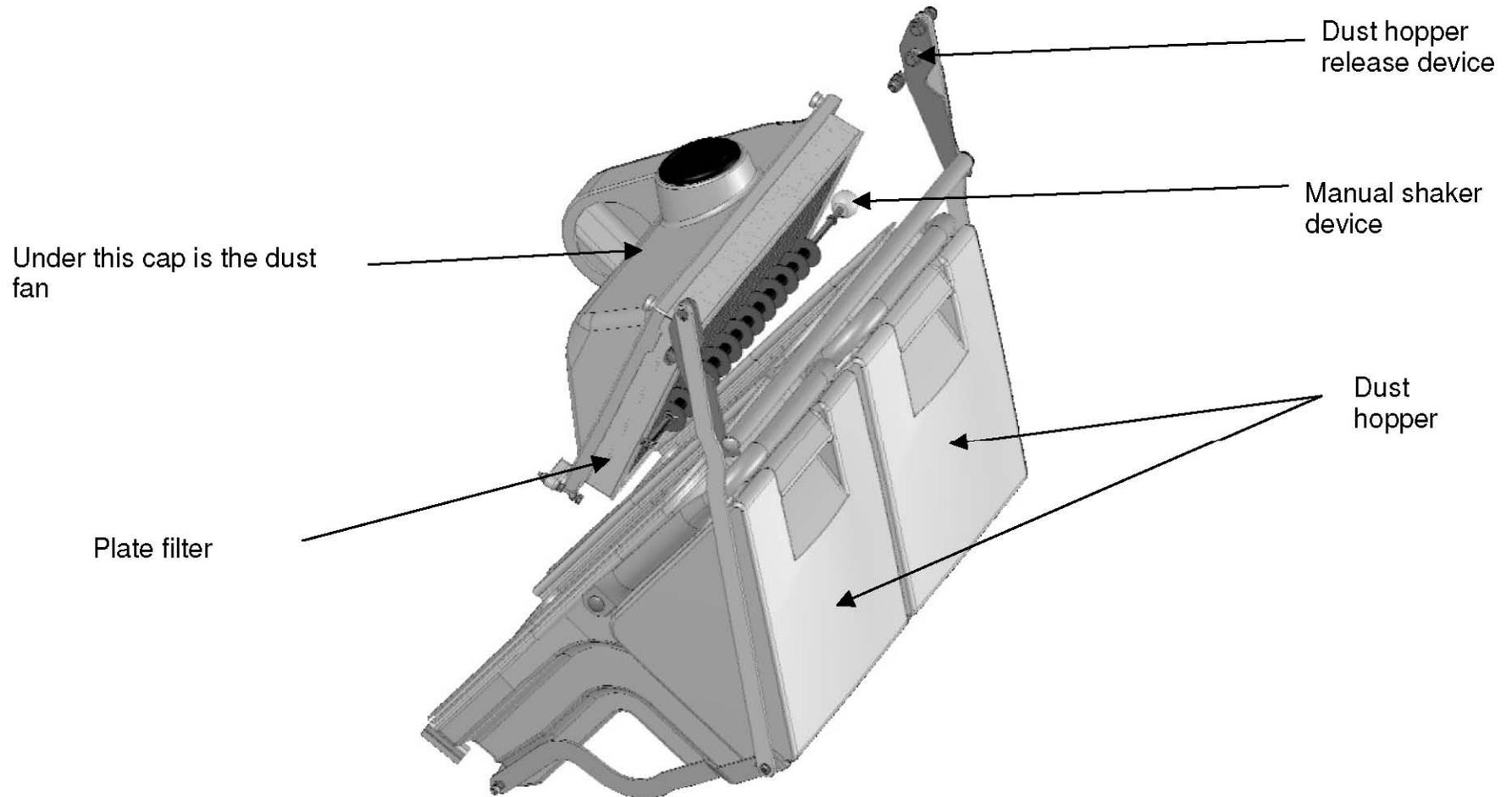
To reach the fan and panel filter, you will have to open the seat cover and then remove the cap.
